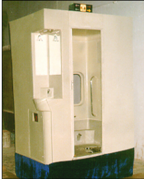
Figure M11.29: Modular FRP toilets for railway coaches
